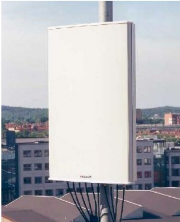
GSM 900 multi-beam antenna array from Ericsson
