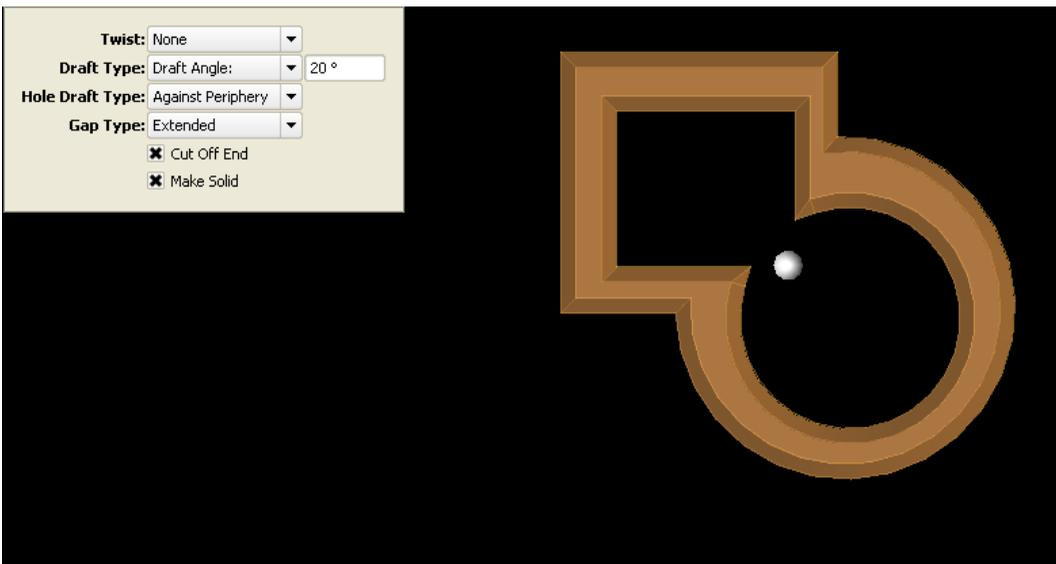
Figure A.49: 3-D Illustration of the Extended gap type
