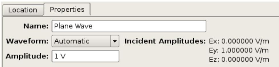
Figure 7.43: The Properties Tab of the Plane Wave Editor
