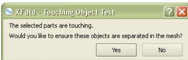
Figure 8.27: The Touching Object Test dialog
