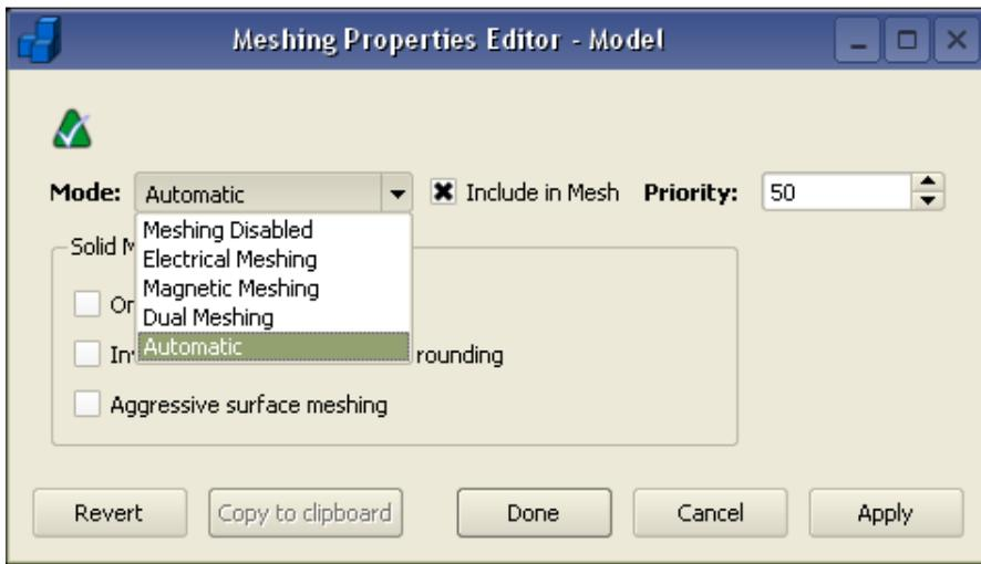
Figure 8.18: The Meshing Properties Editor for a model part
