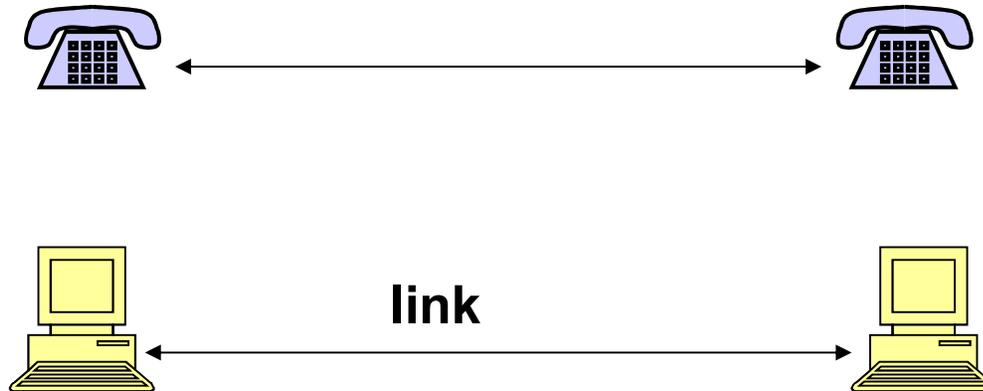
**The communication link can be anything from a simple pair of copper wires, through coaxial cables, radio waves, up to optical fibres.**
