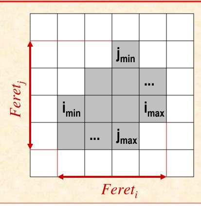
$Feret_{i} = \max(i_{k} - i_{l}), k, l = 1, 2, ..., P$   $Feret_{j} = \max(j_{k} - j_{l}), k, l = 1, 2, ..., P$  P - number of object pixels
