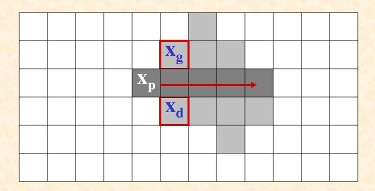
Coordinates  $x_g$ ,  $x_d$ , are stored and filled after finishing with first filled row etc.
