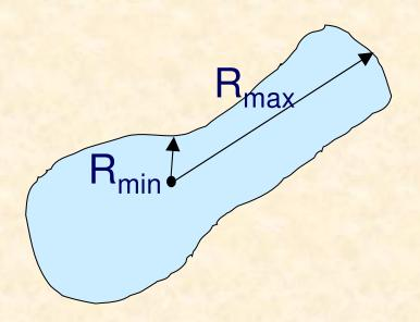
Radii  $R_{min}$ ,  $R_{max}$  are the minimum and maximum distances, respectively, to the boundary from the centre of region mass. The ratio  $R_{max}/R_{min}$  (sometimes called object aspect ratio).
