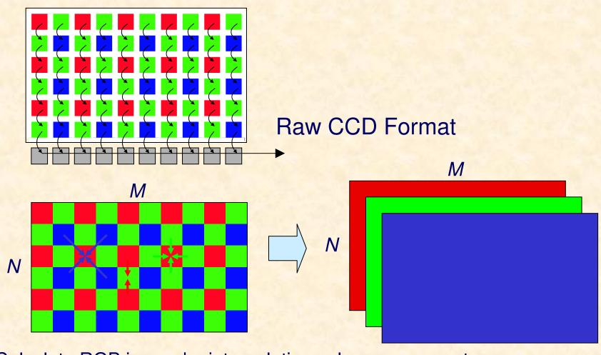
Calculate RGB image by interpolating colour components from the Bayer matrix
