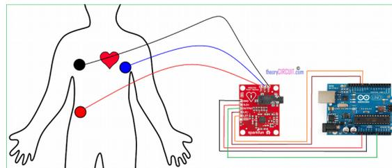
2. ECG signal registration and determination of averaged PR and QT intervals
